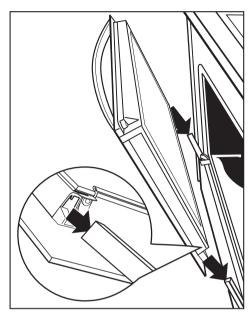
Carefully locate the door over the hinge guides.
